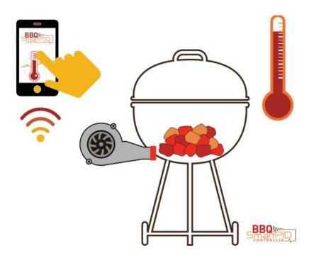
The PID – PWM algorithm will always adjust fan speed in 0-100% range, yet the actual value of rotation speed will be scaled accordingly, depending on MIN/MAX fan speed.
