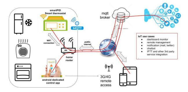
Such architecture allows a number of remote functions using a web app which is manageable by the desktop or mobile browser.
