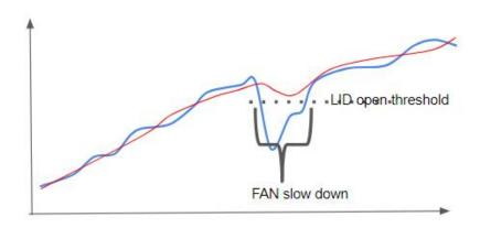
Once finished the LID open timer (or once reached the set point) the fan is reactivated and monitored again by the PID-PWM algorithm.
